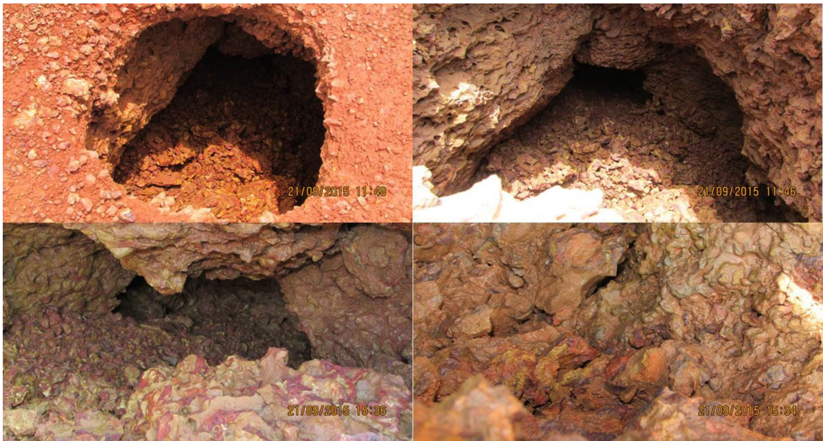
Figure 11 Top surface of soil pipe with internal structure in chronological order at Location 2
