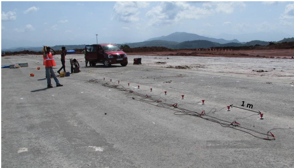
Figure 4 Data acquisition using MASW survey by placing geophones at 1 m spacing
